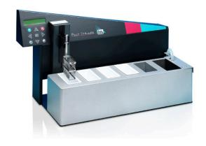
The Poly Stainer™ is the latest innovation in automatic staining from IUL Instruments and offers convenience, reliability, and consistency for Gram Staining, TB Staining, and several other staining procedures.
