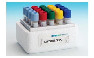
A well-insulated Cryoblock, which can hold up to 20 vials allows operator's to remove a number of vials from the freezer for sub-culture without risk of the culture beads defrosting. The Cryoblock is insulated with a polystýrene shield.
